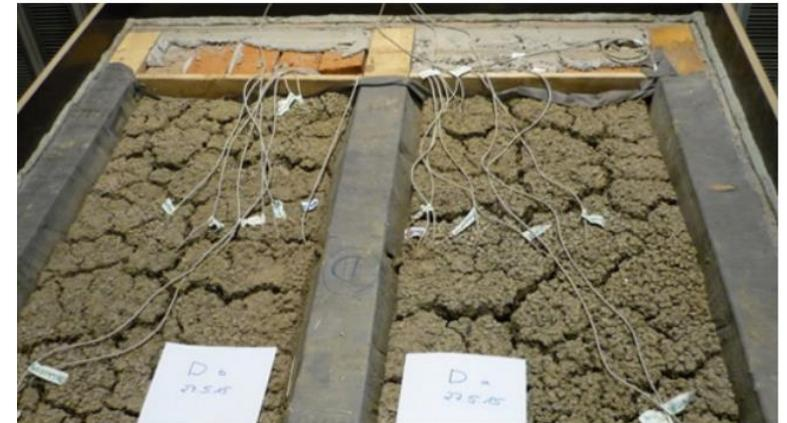
*Wood-beam ceiling with clay filling after five weeks of drying.
